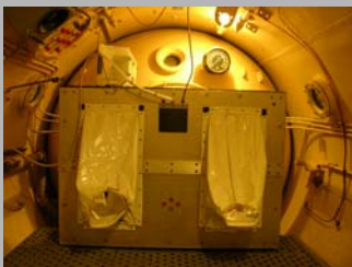
Figure 1. Oxygen delivery system for the UW sheep model in the high pressure Biotron chamber used in DISSUB trials.
